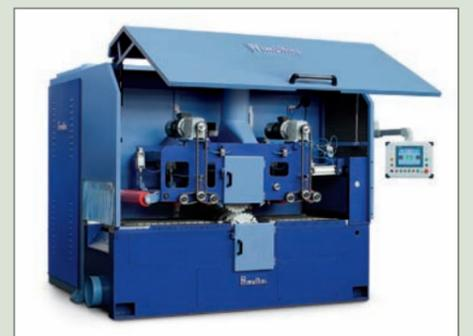
with splinter guards and anti-kickback devices. **Press:** the rollers that make up the press are operated by pneumatic cylinders with adjustable pressure. 10,4 inches touchscreen control panel. ■
